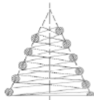
(a) Conical spring.
