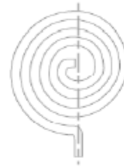
(b) Spiral torsion spring.
